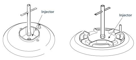
Fig. 7 Auxiliary, rapid and semi-rapid burners
